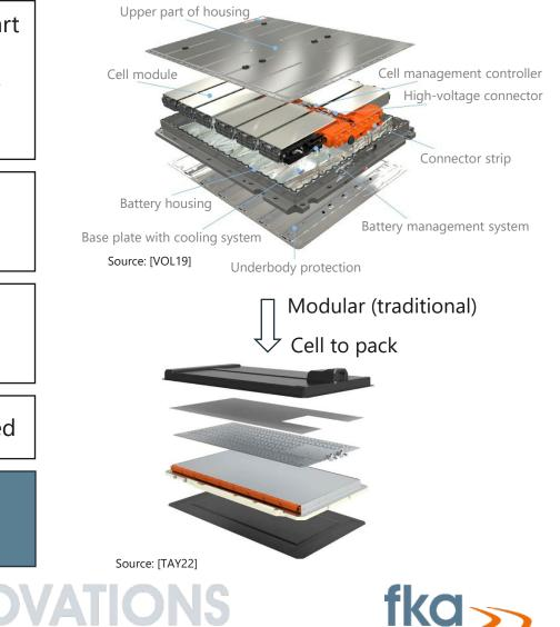
The modular approach "cell to module" (**CTM**) is currently state of the art in automotive industry
