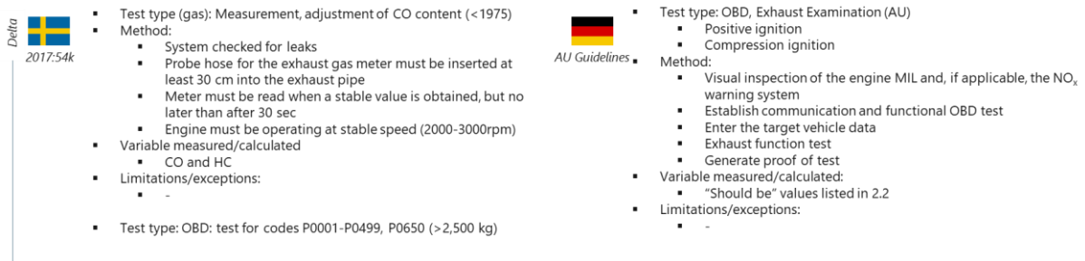
Figure 47: Overview of test procedures for 4-gas analyser
